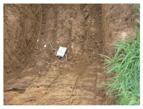
Figure 2: Geothermal meter in situ
